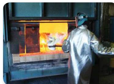
Preheating the ceramic shell
